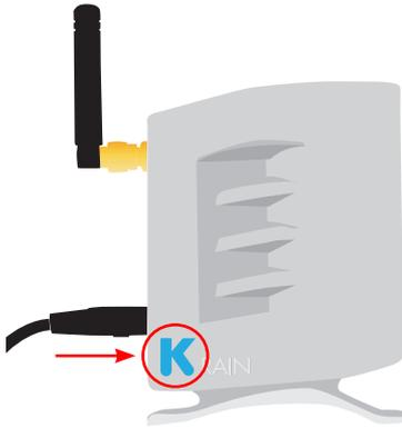
**NOTE:** If the LED is not flashing, reset the hub using the setting button located on the bottom base of the unit. The “K” LED should start flashing (On / Off) after holding down the button for three seconds.
