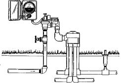
When connecting the lines to the valve outlets, ensure that the correct cam is installed. Install lines to outlets corresponding to numbers on the cam. See diagram for proper zone hookup of outlets.
