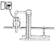
Pump Fed Applications: The 4000 Series Indexing Valve can be installed directly off the discharge side of the pump. The valve is cycled as the pump is turned off and on. It is important to install the valve as close to the pump as possible.
