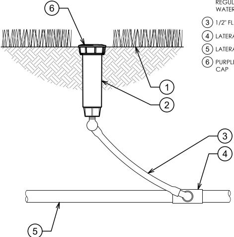
K-RAIN PRO-S SPRAY MODEL 78004-PR30-RCW: 4" POP-UP SPRAY WITH 30 PSI **REGULATOR AND RECLAIMED** WATER CAP
