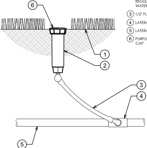
K-RAIN PRO-S SPRAY MODEL 78004-PR40-RCW: 4" POP-UP SPRAY WITH 40 PSI **REGULATOR AND RECLAIMED** WATER CAP
