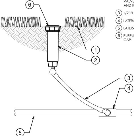
K-RAIN PRO-S SPRAY MODEL 78004-CV-PR30-RCW: 4" POP-UP SPRAY WITH CHECK VALVE, 30 PSI REGULATOR, AND RECLAIMED WATER CAP
