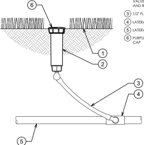
K-RAIN PRO-S SPRAY MODEL 78004-CV-PR40-RCW: 4" POP-UP SPRAY WITH CHECK VALVE, 40 PSI REGULATOR, AND RECLAIMED WATER CAP
