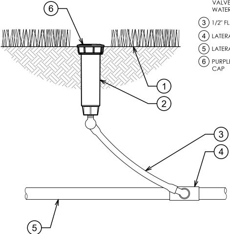
K-RAIN PRO-S SPRAY MODEL 78004-CV-RCW: 4" POP-UP SPRAY WITH CHECK VALVE AND RECLAIMED WATER CAP
